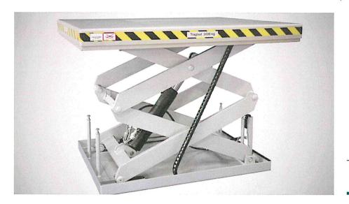
2 TONNEN HUBTISCH VON FLEXLIFT. (FOTO: FLEXLIFT)
